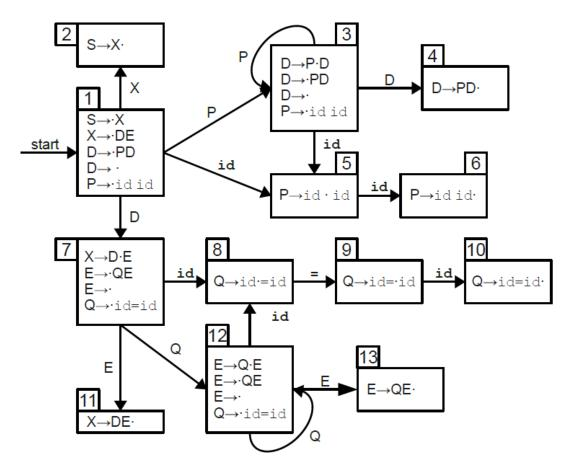
The terminals in the grammar are id, =,\$ where \$ is the end of input symbol.
